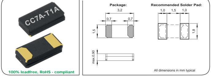
Ultra miniature suitable for implantable medical application SMT ceramic package package height 0.9 mm add 0.75mm on request Fundamental mode up to 50MHz Ind. and Ext. temperature ranges High stability and low aging High shock and vibration resistance Hermetically sealed Ultra low MSL Excellent solderability Swiss made quality Customer specification on request
